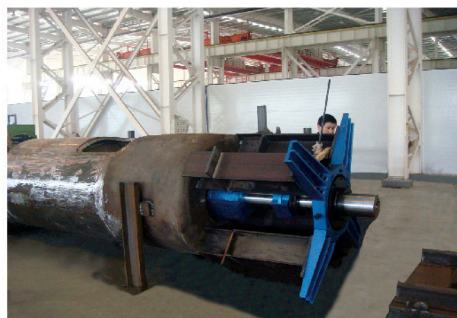
舵叶镗孔 Boring of rudder blade
