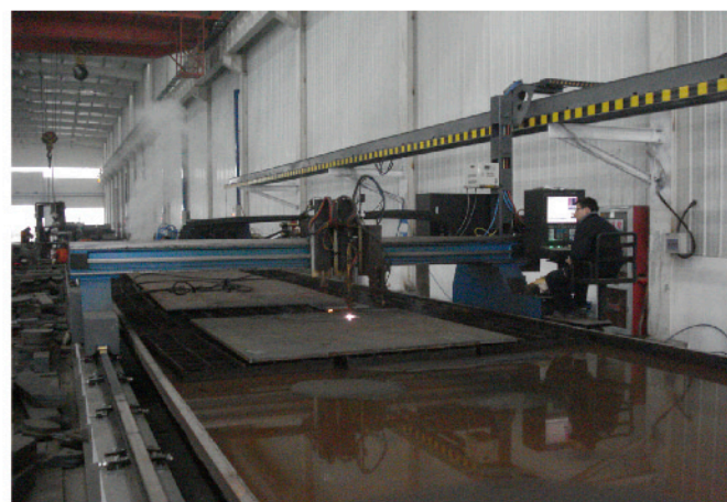
钢板切割 Steel plate cutting
