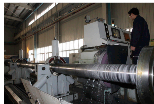
精加工长轴 Finish machining of long shaft
