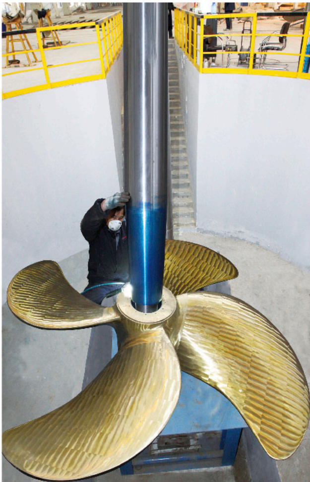
桨轴拂配 Propeller shaft fitting
