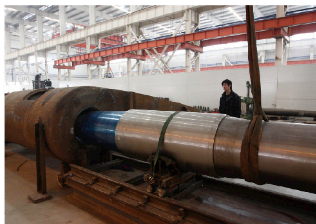
舵叶拂配 Rudder blade fitting
