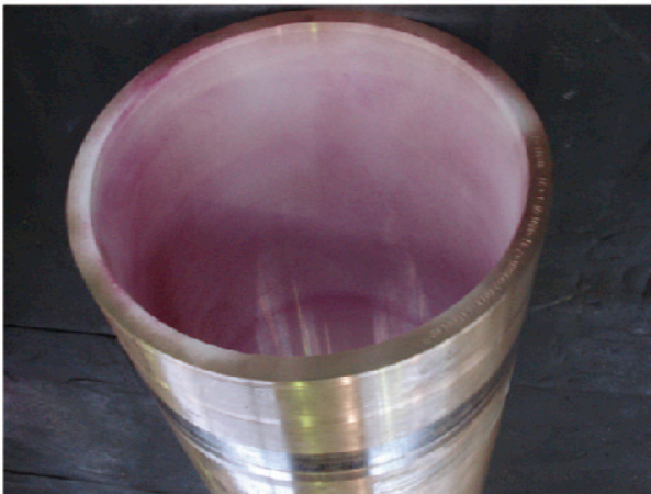
轴套着色探伤 PT test to shaft bush
