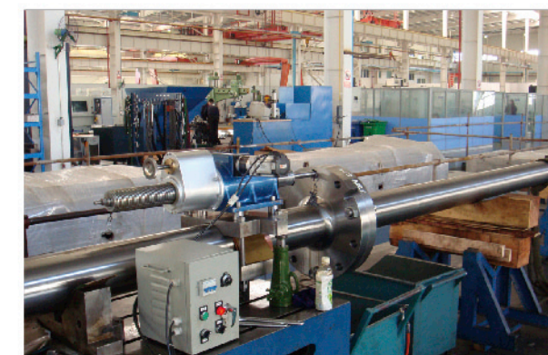
法兰孔配铰 Reaming of flange hole
