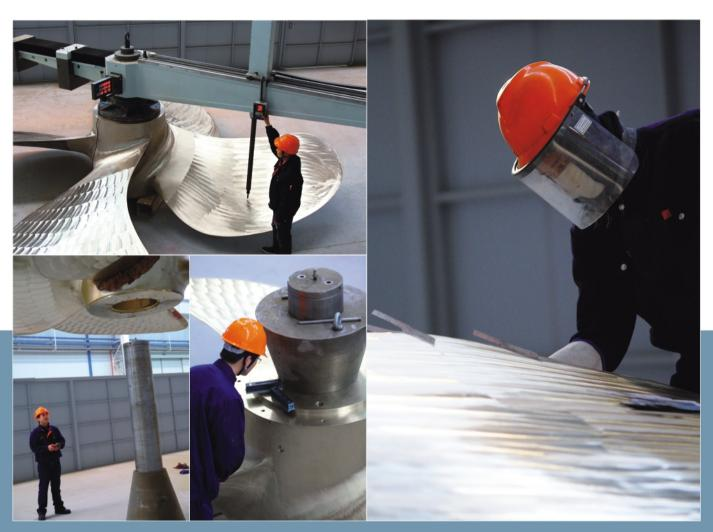
Zhenjiang Tongzhou Propeller Co., Ltd. is staffed with a skilled and experienced team of technicians, who work diligently and use advanced grinding & polishing tools and digital -display three-coordinate measuring instrument to ensure the geometric shape and the appearance quality of the product.
